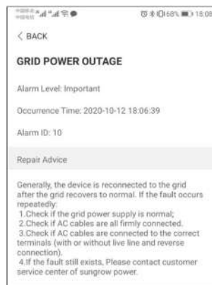
figure 7-9 Detailed Fault Alarm Information
